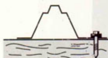
Valley Fixing to Timber
