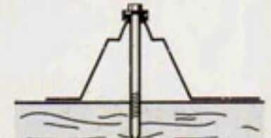
Crest Fixing to Timber
