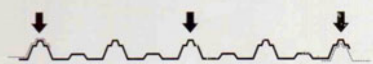
Crest Fixing to steel
